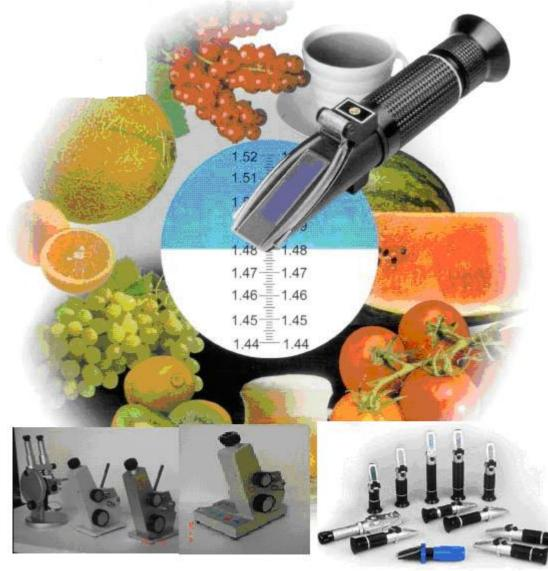
A refractometer is an instrument the concentration of aqueous solution by measuring it's refractive index. All water-based solution can make light bend. The bending of light increases at a rate proportional to the increasing solution concentration.
