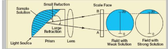
The prism in the refractometer has a greater refractive index than the solution. Measurements are read at the point where the prism and solution meet. With a low concentration solution, the refractive index of the prism is much greater than that of the sample, creating a large refraction angle and a low reading ("A" on diagram). The reverse would happen with a high concentration solution ("B" on diagram).
